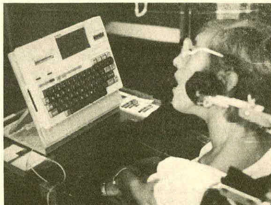
Figure 1. Scanning Portable Anticipatory Communication Aid configured on the Epson HX-20 computer.
