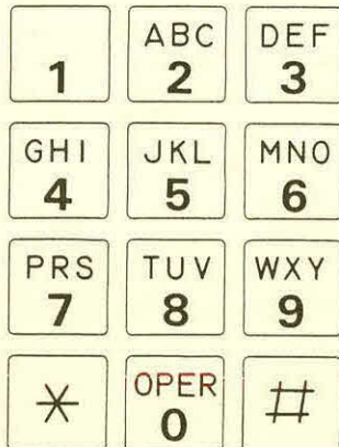
Figure 1. A diagram of the standard Touch-Tone keypad.
