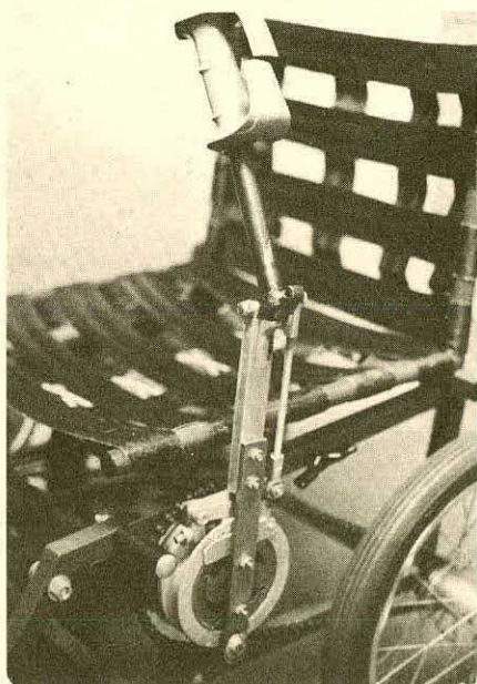
Figure 2 The UVa lever drive system showing the inward motion of the lever that engages the clutch.
