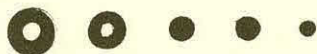
Figure 1. Code for use on a light colored item. The 5 symbol code reads from the largest symbol as 00111. The code must contain 2 zeros as a self check and so a single code group can distinguish 10 items.
